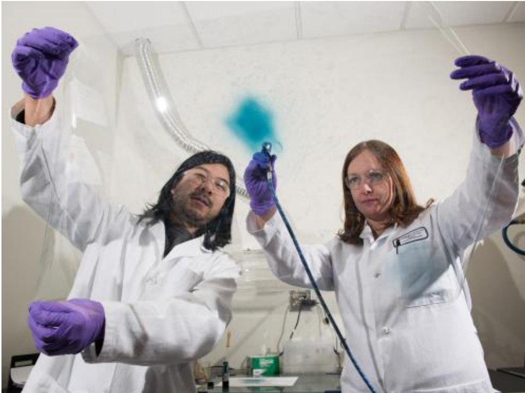
Researchers Eric Shen and Anna Osterholm demonstrate how films of electrochromic polymers can be applied to large surfaces. Credit: Rob Felt
