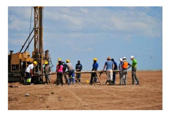
Preparing to remove a core section in its core liner from the lowermost drill rod. Credit: Verena Foerster, University of Potsdam
