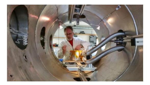
Matthew Sylvest, a doctoral student in space and planetary sciences the the University of Arkansas, adjusts the placement of thermocouples to measure the temperature distribution in the simulated Martian regolith last fall at the Open University in England.
