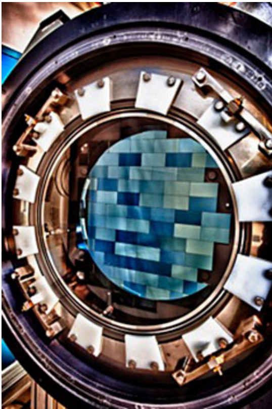
The 570-megapixel Dark Energy Camera.
