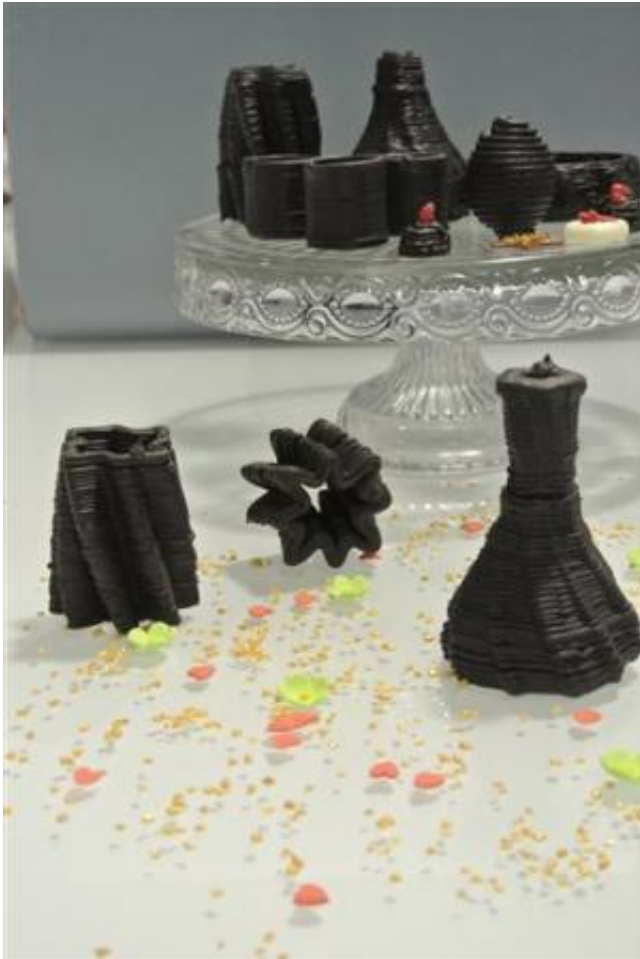
This undated photo provided by Natural Machines on Feb. 5, 2015 shows chocolate shapes made by a food printer. Like more traditional 3-D printers, food printers work by printing out successive layers of edible material. (AP Photo/Natural Machines)
