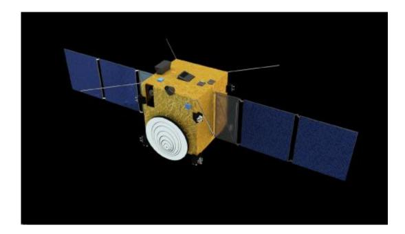
Intended for launch in October 2020, ESA's Asteroid Impact Mission spacecraft will be humanity's first mission to a binary system – the paired Didymos asteroids, which come a comparatively close 11 million km to Earth in 2022. The 800 m-diameter main body is orbited by a 170 m moon. AIM will operate in conjunction with NASA's DART mission to form the international Asteroid Impact and Deflection Assessment mission. Credit: ESA / The Science Office Ltd.
