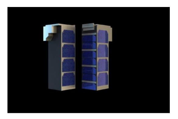
A pair of triple-unit CubeSats. ESA's 2020 Asteroid Impact Mission spacecraft will have room to carry six CubeSat units – potentially single-unit miniature spacecraft but more probably a pair of larger CubeSats as seen here. Credit: ESA / The Science Office Ltd.
