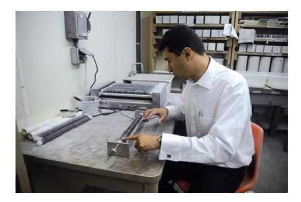
Civil engineer Farshad Rajabipour inspects a tube filled with concrete. The steel frame holding the specimen allows him to measure changes in length of a sealed sample over time. He and his colleagues are working to produce new, environmentally friendly cements with great strength and durability. Credit: Curtis Chan
