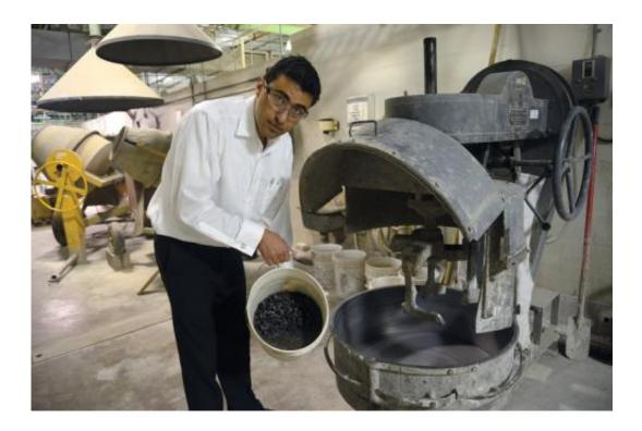
In the Civil Infrastructure Testing and Evaluation Lab at Cato Park, Farshad Rajabipour prepares to add aggregate (crushed rock) to a concrete mixer. The aggregate is dark because it has been soaked in water, one step in a new practice of internal curing of concrete to improve its strength, durability and service life. Credit: Curtis Chan
