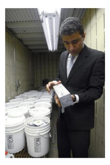
Engineer Farshad Rajabipour examines a concrete prism being used to study the alkali-silica reaction, which is a major cause of deterioration in concrete structures. Behind him, each white bucket holds four such prisms at high humidity and a temperature of 38 degrees Celsius (about 98 degrees Fahrenheit). Researchers measure expansion of the prisms over time and remove slices of them every few months for microscopic examination. Credit: Curtis Chan
