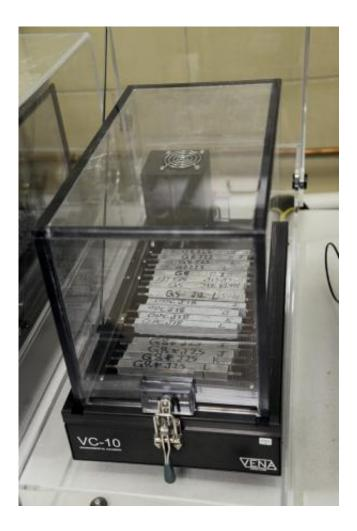
Samples of a new low-energy, low- CO2 concrete made using coal combustion ash instead of Portland cement. The samples are in an environmental chamber that allows researchers to vary the temperature and humidity in order to study the concrete's shrinkage and propensity to crack. Credit: Curtis Chan
