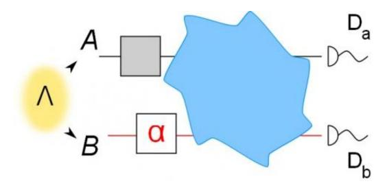
An illustration of the delayed-choice experiment, which shows that a photon exhibits both particle and wave behaviors. The physicists used this experiment to show that seemingly reasonable classical assumptions may not be so reasonable after all. Credit: Ionicioiu, et al. ©2015 American Physical Society
