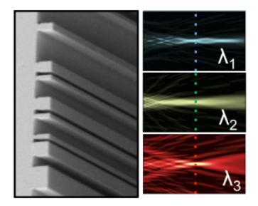
This completely flat, ultrathin lens can focus different wavelengths of light at the same point, achieving instant color correction in one extremely thin, miniaturized device. Credit: Federico Capasso and Francesco Aieta, Harvard SEAS
