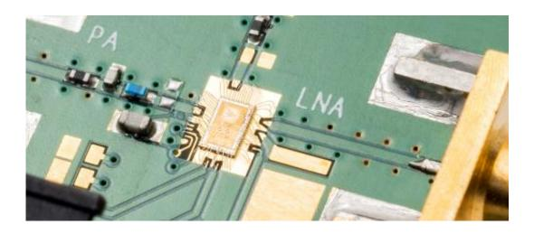
Electrical-Balance Duplexer in 0.18µm SOI CMOS
