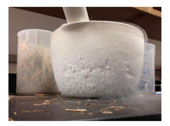
Biomass being crushed using liquid nitrogen causes ice to form outside the bowl. The researchers later realized that crushing the biomass in these conditions was unnecessary. Credit: Timothy A. Kremer, Indiana University
