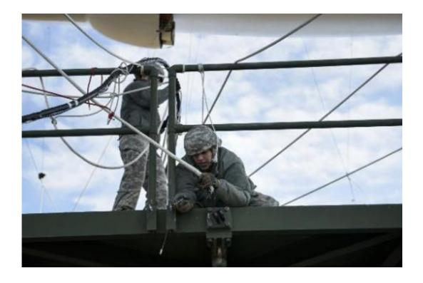
Soldiers secure a line while mooring an aerostat to its mobile mooring station at the Aberdeen Proving Ground in Maryland
