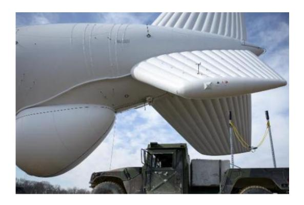
A Humvee with a makeshift slingshot used to remove snow and ice from an aerostat is seen at the Aberdeen Proving Ground in Maryland
