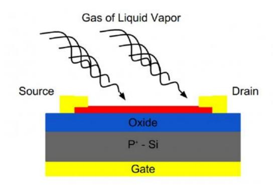
Schematic of the molybdenum disulfide (MoS2) thin-film sensor with the deposited molecules that create additional charge. Credit: UC Riverside
