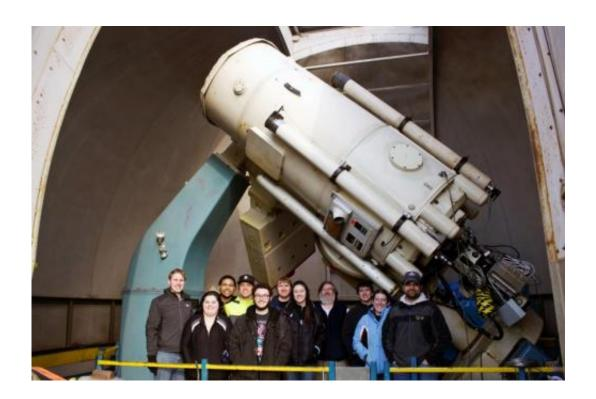
The University of Toledo observing team poses with the HPOL instrument (far right) mounted on the Ritter Observatory 1-m telescope. Graduate and undergraduate students in the Department of Physics & Astronomy conduct observations with HPOL every clear night. Credit: Kevin Hardegree-Ullman
