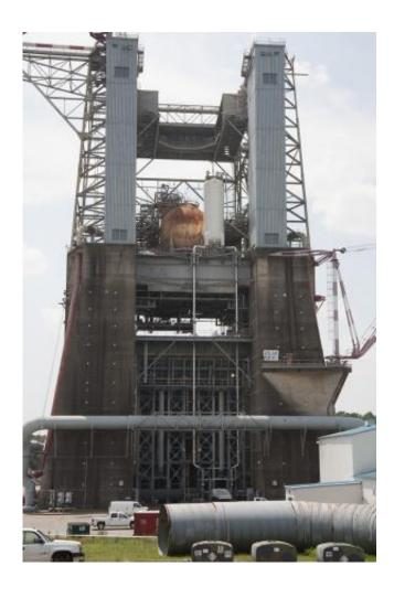
A full-scale replica of the SLS liquid oxygen tank feed system is set up on one of the Marshall Center's test stands for anti-geyser testing.
