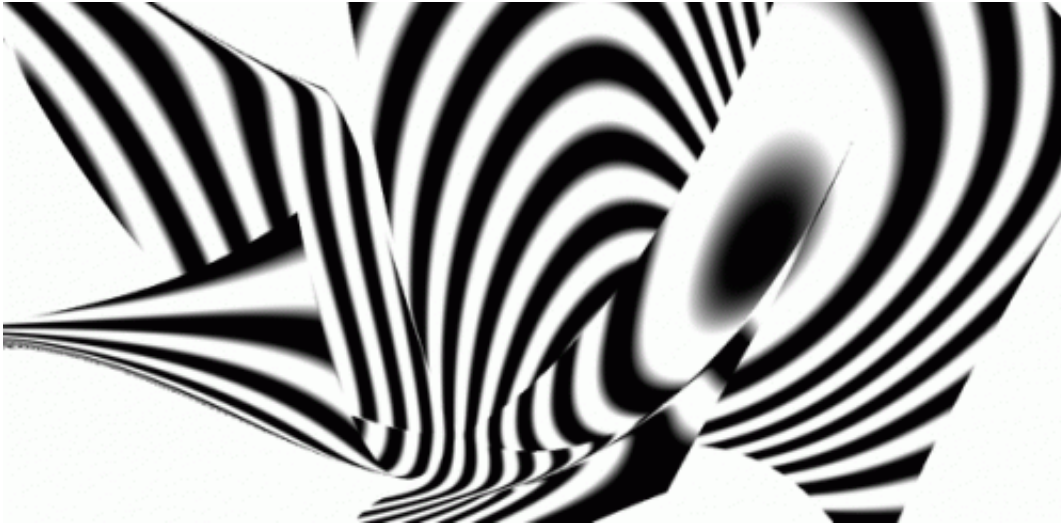
Reflection lines on a creased structure. Credit: Jirí Kosinka
