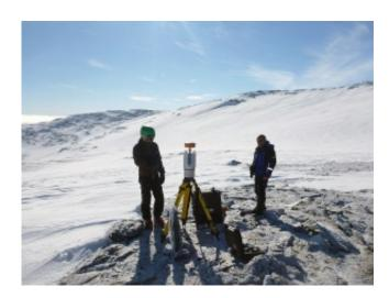
Laser scanning the Kringsollfonna ice patch to measure how much snow accumulates in the winter and melts in the summer. Credit: Geir Vatne, NTNU
