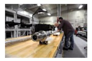
Accident-tolerant fuel test samples are prepared for irradiation at INL's Advanced Test Reactor Test Train Assembly Facility.
