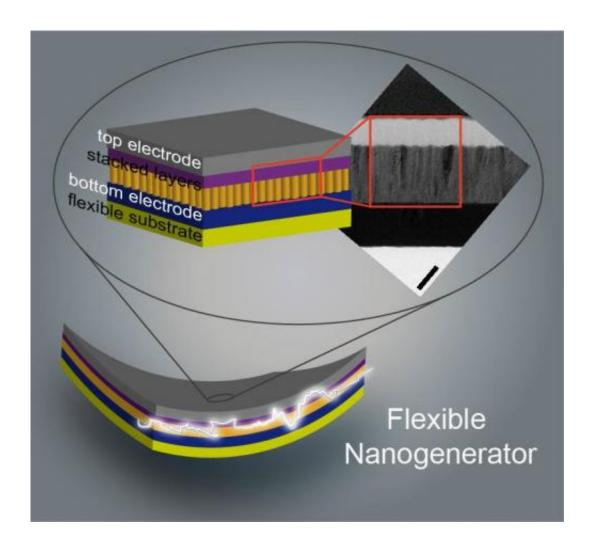
This illustration shows stacked flexible nanogenerators (left), and a cross-sectional transmission electron microscopy image of the ZnO/AlN-stacked structure. The scale bar on the right represents 200 nm. Credit: Giwan Yoon/Korea Advanced Institute of Science and Technology
