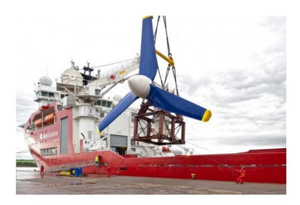
Tidal turbines such as the one pictured here will be used to convert the energy of the tides into useful forms of power, mainly electricity. Credit: FORCE
