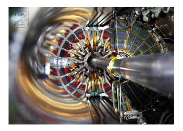
The Compact Muon Solenoid (CMS) pixel detector. The CMS is used to detect particles generated by collisions at the Large Hadron Collider particle accelerator. A University at Buffalo team is working to connect findings from particle acceleration experiments to findings in cosmology. Credit: CERN
