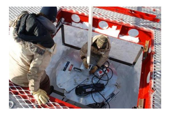
WISSARD drillers set in place an ultraviolet light collar, used for purification, at the borehole site near the Whillans Ice Stream grounding zone in Antarctica. Credit: Frank Rack, UNL Science Management Office
