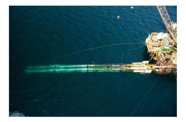
The pipelines were found to sink into "shoulders" of solid seabed on either side of the spanned space, creating further stability by anchoring the pipe. Credit: Shell
