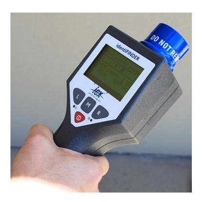
A handheld radiation identifier, such as that pictured here, connected to the SIP would respond just as if a real radiation source were present.
