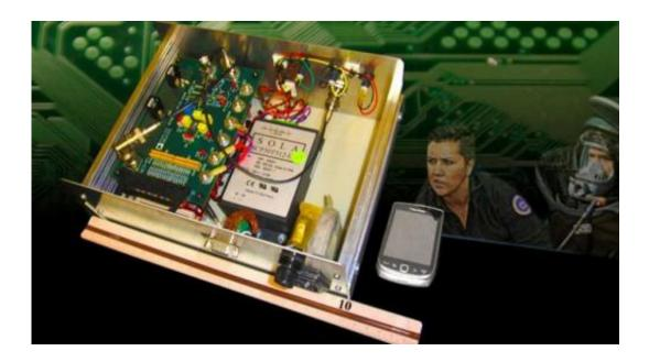
The LLNL Spectroscopic Injection Pulser prototype directly injects signals into radiation detection equipment, exactly like a real radiation source. This laboratory-scale prototype will support miniaturization to something near the size of a cellphone.
