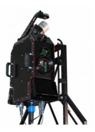
Essess' thermal-imaging rig, mounted on a car's roof, includes long-wave infrared radiometric cameras, near-infrared cameras, and a LiDAR system to capture 3-D images. An onboard control system has software to track the route and manage the cameras.
