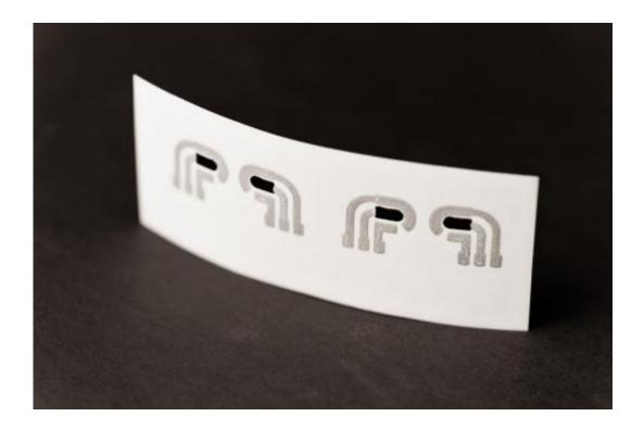
The device consists of carefully patterned electrodes printed on temporary tattoo paper. Credit: Jacobs School of Engineering/UC San Diego
