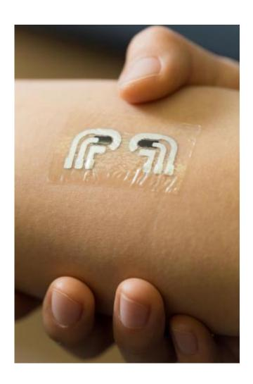
Nanoengineers at the University of California, San Diego have tested a temporary tattoo that both extracts and measures the level of glucose in the fluid in between skin cells. The device is flexible and easy to wear. Credit: Jacobs School of Engineering/UC San Diego
