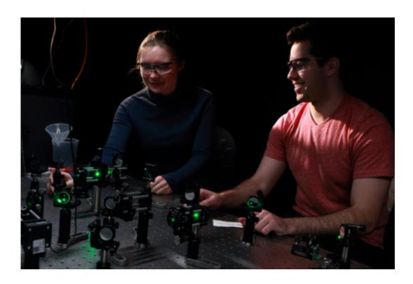
A. Jolene Mork, a fifth-year MIT graduate student in chemistry, and Mark C. Weidman, a fourth-year MIT chemical engineering graduate student, work with an array of mirrors and lenses coupled to a laser that directs a light beam to a microscope (not shown) for carrying out time-resolved photoluminescence spectroscopy experiments in the Tisdale Lab at MIT. Credit: Denis Paiste/Materials Processing Center
