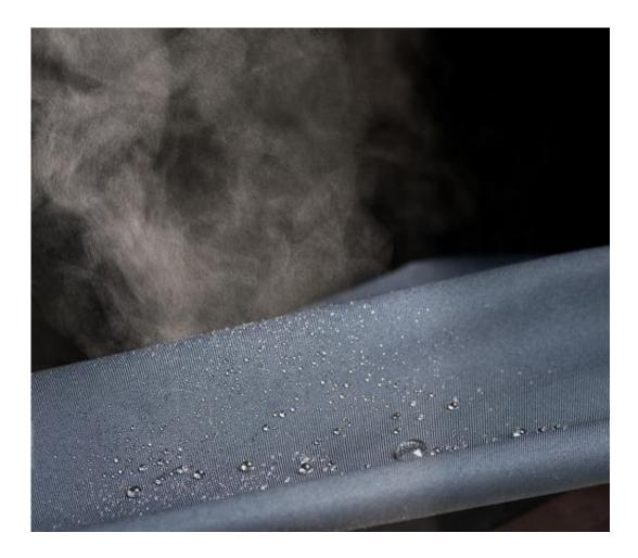
Breathable fabric used in field test traps waste and allows only tiny water vapor molecules through. Credit: Evan Krape, University of Delaware
