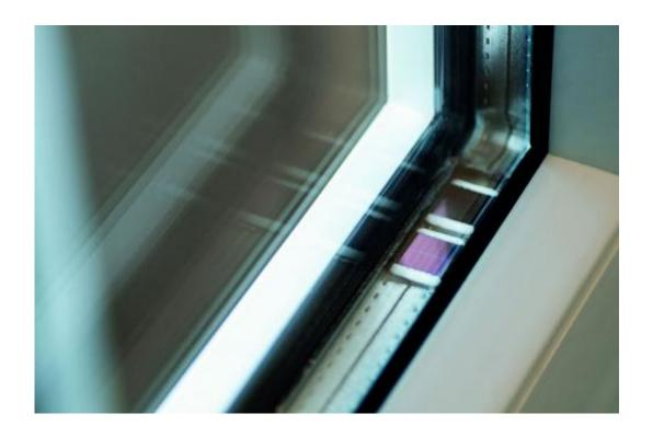
The chip affixed to the window frame supplies itself with energy. Credit: Fraunhofer IMS
