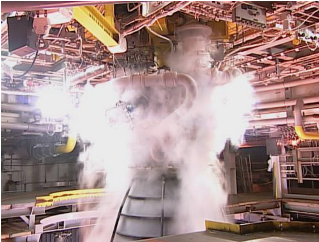
A close-up view of the RS-25 engine from the test stand. Credit: NASA
