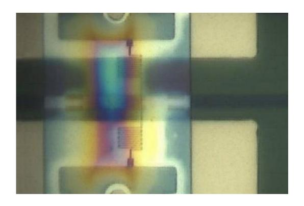
One of the researchers' new photon detectors, deposited athwart a light channel — or "waveguide" (horizontal black band) — on a silicon optical chip. Credit: Nature Communications
