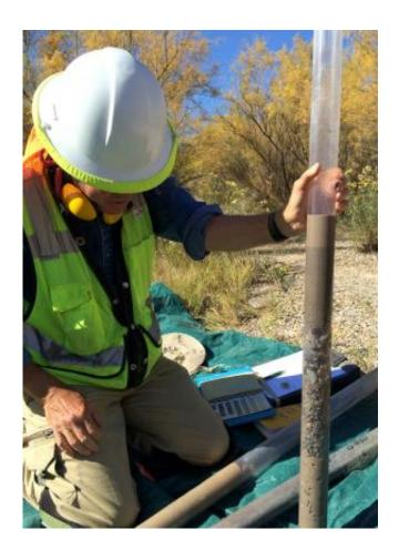
The team drills into contaminated sediments at the Naturita site, Colorado, to collect samples from various depths. Zones rich in organic material, which are believed to be a major factor in trapping uranium contamination, are generally found 10 to 30 feet below the surface. Credit: John Bargar/SLAC National Accelerator Laboratory
