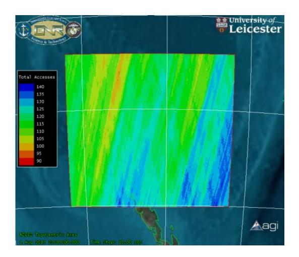
The computer model generated by the authors represents a rectangular zone of ocean off the north coast of New Zealand approximately 1000 x 1000 km in size. The model is used to calculate how many satellite sensors capture a target in the zone, what detail they provide, and how often the point is revisited, represented by coloured plots. The scientists then use the results of this model to estimate how the system would work on a global scale.
