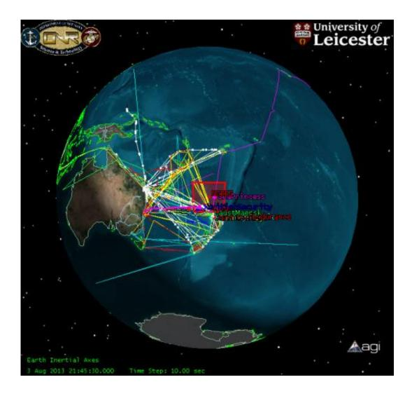
The authors used real vessel track data to reproduce the voyages of ships in the ocean around New Zealand. The computer model was then used to calculate how often each would be detected from space, and how accurately the paths of these vessels would be followed. More accurate tracking would lead to reduced search zones and faster recovery in the event of an accident at sea."
