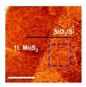
Two-dimensional (2D) materials such as molybdenum-disulfide (MoS<sub>2</sub>) are attracting much attention for future electronic and photonic applications ranging from high-performance computing to flexible and pervasive sensors and optoelectronics. But in order for their promise to be realized, scientists need to understand how the performance of devices made with 2D materials is affected by different kinds of metal electrical contacts.
