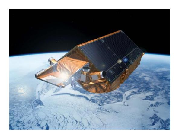
The CryoSat mission provides data to determine the precise rate of change in the thickness of the polar ice sheets and floating sea ice. It is capable of detecting changes as little as 1 cm per year. The information from CryoSat is leading to a better understanding of how the volume of ice on Earth is changing and, in turn, a better appreciation of how ice and climate are linked. Credit: ESA – P. Carril
