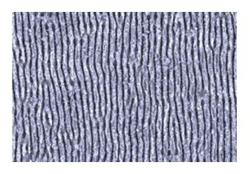
Scanning electron micrograph showing a ripple pattern formed on a silicon surface using a femtosecond laser beam. This surface absorbs more light than an unprocessed surface and could enhance solar cell efficiency. Credit: Elsevier
