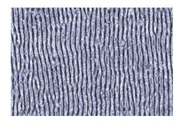
Scanning electron micrograph showing a ripple pattern formed on a silicon surface using a femtosecond laser beam. This surface absorbs more light than an unprocessed surface and could enhance solar cell efficiency. Credit: Elsevier
