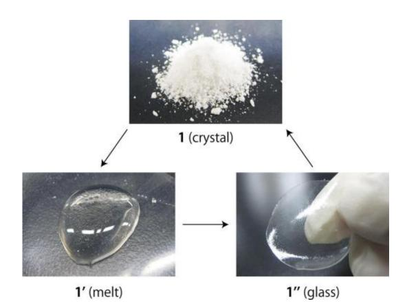
Scientists have discovered that some coordination polymers (CPs) undergo a reversible solid-liquid phase transition as the temperature changes. Shown here are the crystalline (solid) state, the molten (liquid) state, and the glassy (supercooled) state of a CP. Credit: Umeyama, et al. ©2015 American Chemical Society
