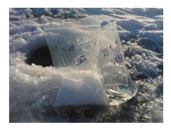
Freezing technology can be utilised in waste water treatment. When waste water freezes, it is purified through the formation of a cleaner layer of ice. The clean layer of ice can be removed from the rest of the waste water, and the remaining waste water is more concentrated. The new energy-efficient method of purification is based on the natural freezing process of water: energy is required only for breaking the ice
