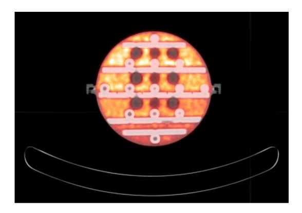
A fused PET-CT image of the new phantom with its traceably calibrated amount of fluorine-18 (orange). The circular objects are the MR-visible test spheres; in this PET-CT image they appear as regions with no PET response.
