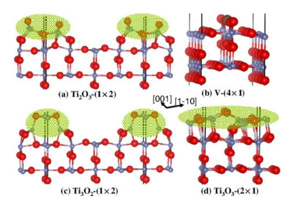
Side views of stable structures of rutile TiO2(110): (a) Ti2O3- $(1\times2)$ , previously proposed in Refs. [7,9], (b) V- $(4\times1)$ , (d) Ti3O3- $(2\times1)$ , as well as (c) metastable Ti3O2- $(1\times2)$ . Ti and O atoms are represented by small gray and big red balls, respectively. An O vacancy in V- $(4\times1)$  is represented by the dark gray ball. Structural features are highlighted by yellow shades Credit: Qinggao Wang
