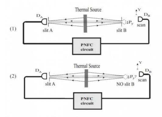
Illustration of Popper's experiment realized with randomly paired photons in a thermal state. In the second set-up, there is no "slit B" for the photon on the right. The new results show that this photon is not affected by a measurement on the left photon (which does travel through a slit), in agreement with Popper's prediction. Credit: Tao Peng, et al. ©2015 EPLA
