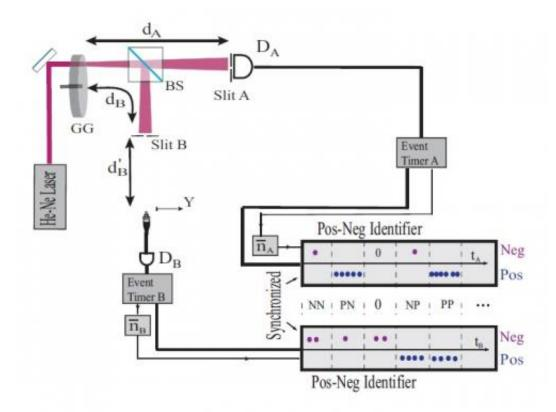
Illustration of the new experimental set-up used to realize Popper's experiment. One entangled photon travels through slit A, while the other travels a different path through slit B, which can be adjusted to be the same width as slit A or wide open. Credit: Tao Peng, et al. ©2015 EPLA
