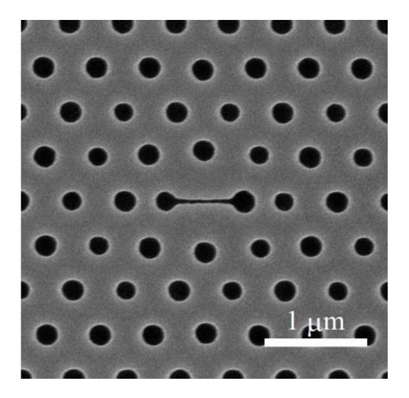
Top view of the group's nanolaser, in which the center narrow slot (horizontal line) is the main part of the sensor. The periodic holes form a photonic crystal, and although the size of the holes appears to fluctuate they've been intentionally modified so the laser's emission is effectively extracted to the top. Credit:
