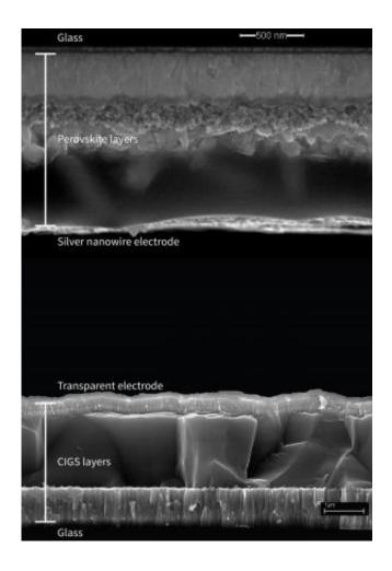
Microscopic cross-section of a tandem solar cell made with two photovoltaic materials, perovskite and copper indium gallium diselenide, or CIGS. Credit: Colin Bailie, Stanford University
