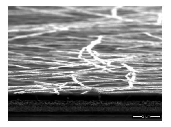
Microscopic image of a perovskite solar cell with a silver nanowire mesh that enables semi-transparency. The perovskite cell is mechanically stacked onto a conventional silicon cell to enhance efficiency. Credit: Colin Bailie, Stanford University
