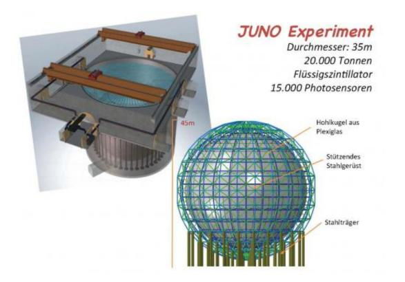
Schematic depiction of the JUNO detector showing the shielded acrylic sphere (lower right). The detector is surrounded by a pool of water to protect it against background radiation (upper left). Credit: Michael Wurm
