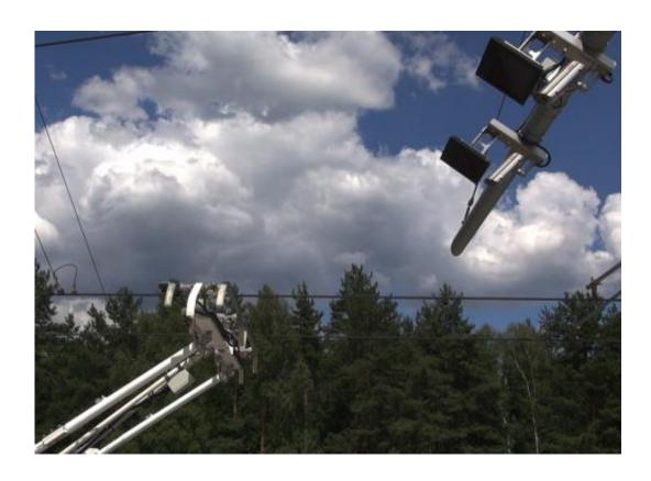
Siemens is developing an automatic monitoring system for pantographs. Designed initially for electric and hybrid trucks on eHighways, the system uses cameras and sensors to check the condition of pantographs in order to prevent damage to the overhead contact wire. Similar but much more complex systems are occasionally used for electric trains.
