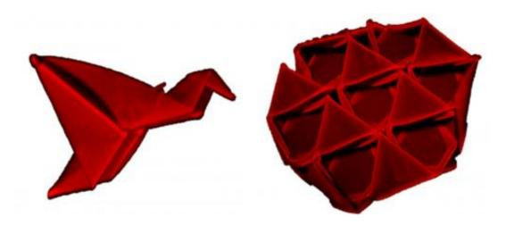
These are three-dimensional reconstructions (from confocal fluorescence microscopy) of self-folded origami structures with overall dimensions slightly below 1 mm. At left is a bird based on the design "New Flapping Bird" by Randlett, and at right an octahedron-tetrahedron ('octet') truss design independently discovered by many origamists including Huffman, Kawasaki and Resch. Credit: UMass Amherst
