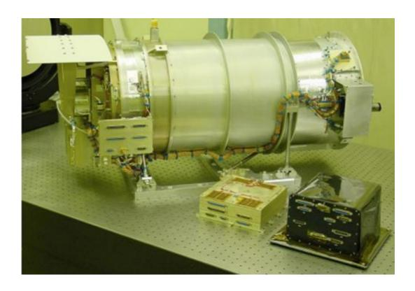
EPIC instrument views the entire sunlit face of the Earth from sunrise to sunset in 10 narrowband channels, from ultraviolet to near infrared. These measurements can be used to determine ozone, aerosols, cloud heights, dust, volcanic ash. Credit: NASA / DSCOVR
