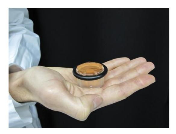
Glucolight's measuring head with the smart membrane. Credit: Empa
