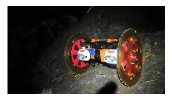
VolcanoBot 1, shown here in a lava tube -- a structure formed by lava -- explored the Kilauea volcano in Hawaii in May 2014. The robot is enabling researchers at NASA's Jet Propulsion Laboratory to put together a 3-D map of the fissure. Credit: NASA/JPL-Caltech
