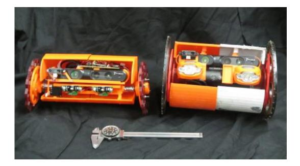
Two robots designed to explore volcanoes are pictured here. VolcanoBot 1 (right) has a length of 12 inches (30 centimeters) and 6.7-inch (17-centimeter)
