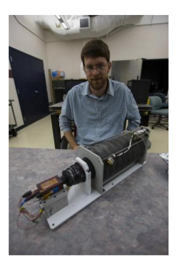
Wallops engineer Scott Heatwole and his team are developing a precision attitude sensor or star tracker that would be able to locate points of reference, or, in other words, stars, during daylight hours. Heatwole specifically developed the technology for the Wallops Arc Second Pointer. Credit: Patrick Black/NASA
